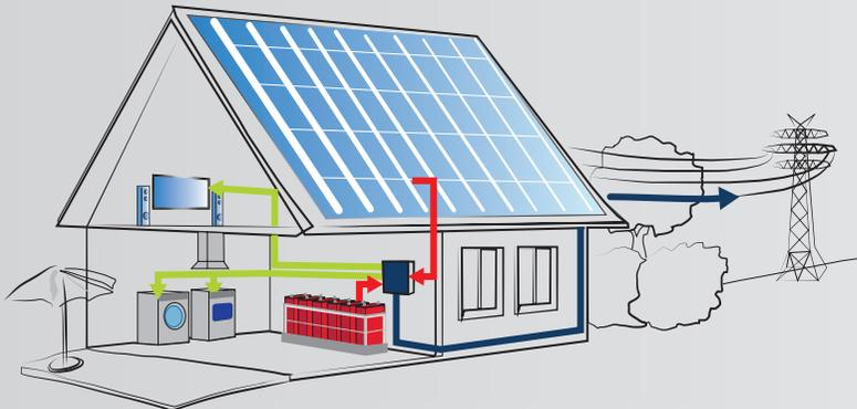
Electrical power generated by the sun and/or wind, and actual power consumption never match. The result is feedback of power into the grid when excess power is generated, and power needed from the grid when power generation is insufficient.
